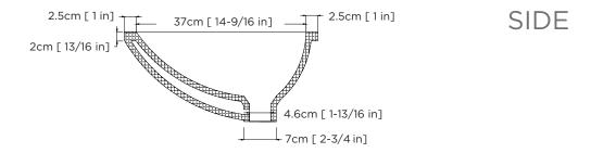
By IAPMO, ceramic lavatory warpage is defective only if warpage of flat slab out of horizontal plane exceeds 6.3 mm/m (0.25 in/ft) on all sizesOR warpage on back of lavatories that are attached to the wall exceeds 3 mm (0.13 in).
