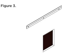
**Step 5:** Secure the cleat in the back of the mirror to the wall cleat. Hide all wires in the opening.
