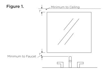
**Step 2:** Determine the location of wall cleat. Make sure to use the leveling tool to ensure the pilot holes are level. Drill 5/16" pilot holes into the wall.
