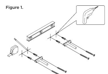
**Step 2:** Install the brackets using the self tap anchors and long screws provided.
