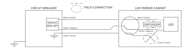
**NOTE:** Locate the wires behind the cabinet. The qualified electrician has the option to hard wire the cabinet, or attach to a pig tail and plug into a wall outlet.
