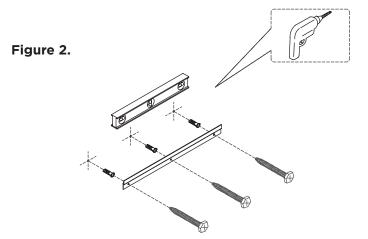
**STEP 3:** Secure the anchors in the wall, and then fasten the screws provided into the anchor to secure the wall cleat.
