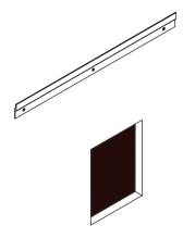
**STEP 5:** Secure the cleat in the back of the mirror to the wall cleat. Hide all wires in the opening.
