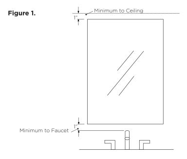
**STEP2:** Determine the location of wall cleat. Make sure to use the leveling tool to ensure the pilot holes are level. Drill 5/16" pilot holes into the wall.
