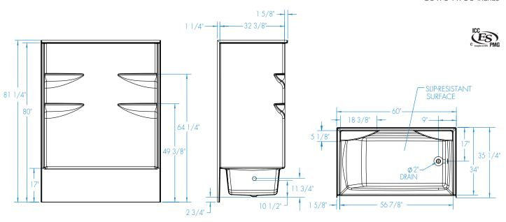
FEATURES lbs Dimensional Tolerance ± 3/8". Dimensions needed for site preparation should be measured from the unit. Aquatic assumes no responsibility for preparatory work.
