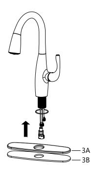
For three-hole installation: Deck plate (3A), base plate (3B), and silicone sealant (optional) are required.
