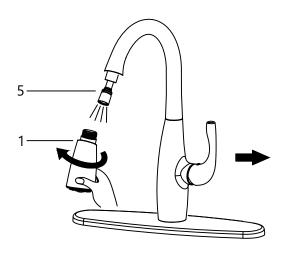
Remove spray head (1) from spray hose (5). Hold tip of spray hose (5). Turn faucet on and let the water run for 60 seconds to flush any debris.
