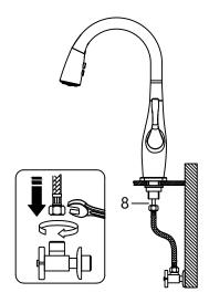
Connect waterlines to hot and cold copper lines (8). Connect waterlines to angle stops.
