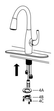
Insert faucet body (2) into hole in countertop or deck plate assembly (3). Install mounting hardware (4A, B & C) from underneath the countertop.
