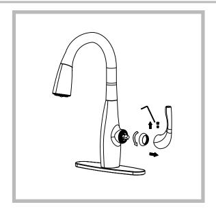
**Step 1:** Remove button located at the top of the handle. Loosen the set screw with a hex wrench. Remove the handle and unscrew cartridge cover by hand.
