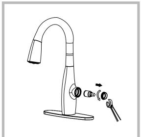
**Step 2:** Unscrew the locking nut with an adjustable wrench. Remove ceramic disc cartridge.
