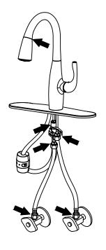
Check for leaks at the connections. Retighten if necessary.
