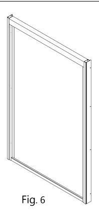
5. Move the assembled frame to the designated position and adjust the **Wall profiles (#02)** so that they are tight to the walls by slightly pulling them out of the **Glass Profiles (#03)** if necessary.
