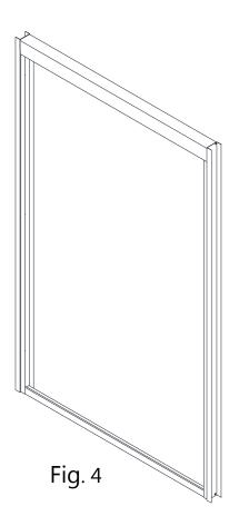
4. Push the **Glass Profiles (#03)** all the way over the **Wall Profiles (#02).** Make sure the Wall Profile flange faces inside the shower.
