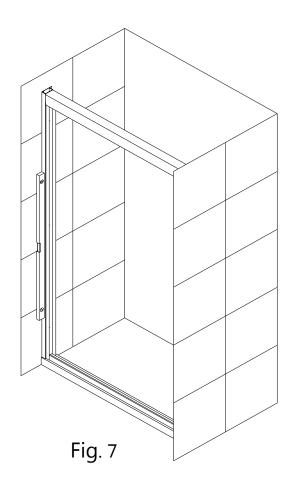
6. Hold the frame in the correct position, mark the drill holes on the wall through the holes on the flange of the Wall Profile (#02).
