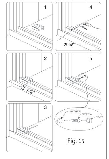
11. Fasten the **Rubber stopper (#14)** inside the groove of the **Wall Profile (#02)** using the **Pan Head screw ST4.2×16 (#08)**. Repeat for all 6 of the **Rubber stoppers (#14).**
