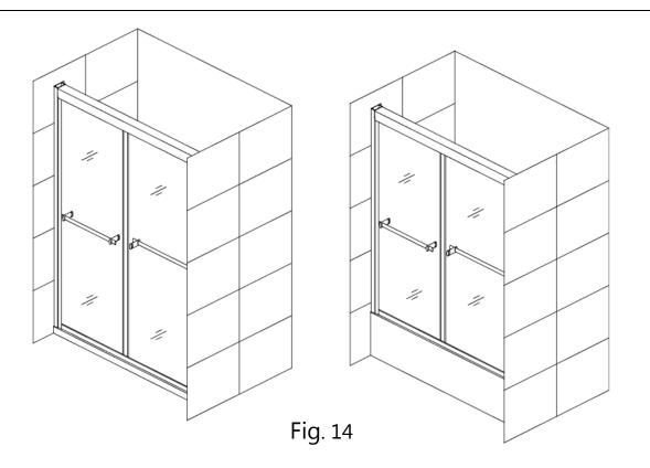
10. From inside the shower, slide both Glass Doors (#01) to the right. Place the Left guide block (#13) to the end of the guide rail and mark the drill hole in the Bottom Guide rail (#04) through the pre-drilled hole on the block using an Ø1/8" drill bit. Drill the hole and secure the Guide block with the Pan Head screw ST4.2×16 (08) using the washers and the Decorative Covers (10). See fig. 15 for details.
