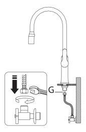
Connect waterlines (G) to copper lines and angle stops. Tighten both ends of waterlines with an adjustable wrench until snug. Turn on angle stops and check for leaks (DO NOT TURN FAUCET ON)
