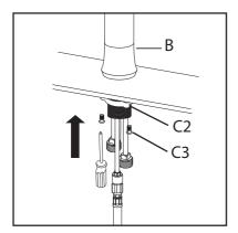
Adjust the direction of faucet body (B). Tighten mounting nut (C2) until snug. Tighten mounting screws (C3) to nut with a Phillips screwdriver until snug
