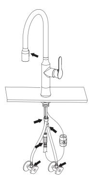
Check for leaks at the connections
