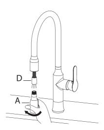
Remove spray head (A) from hose (D). Hold tip of hose (D). Turn faucet on for 60 seconds to flush any debris
