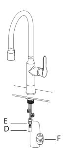
Connect hose (D) to check valve connector (E). Tighten with wrench. Install weight (F) on lowest vertical point on hose (D)
