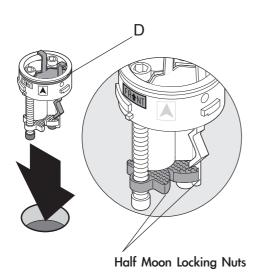
Insert base (D) into sink or countertop with "FR↑NT" facing forward. Tighten screws on base (D) with 4mm hex wrench (J) until base is secure on sink or countertop
