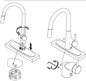
**Note:** "▲" on base should be in alignment with "▼" on faucet body. Rotate faucet counterclockwise to secure on base.
