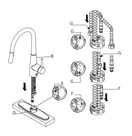
Remove Quick Connect (I) from spray hose (E). Insert spray hose (E) into small hole of base (D). Insert hot & cold waterlines (G) and supply hose (F), one by one, in large hole of base
