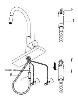
Attach Quick Connect (I) to spray hose (E). Attach the other end onto the supply hose (F) until you hear a click
