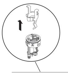
Installer Tip: Rotate the two half-moon shaped locking nuts inward before inserting base (D) into deck plate (C)
