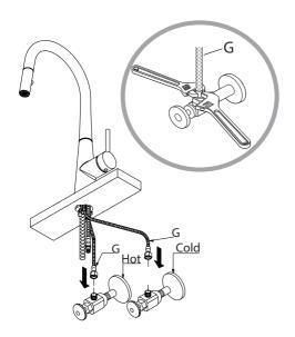
Thread hot & cold waterlines (G) onto angle stops. Tighten with adjustable wrench until snug. Turn on the angle stops and check for leaks (DO NOT TURN FAUCET ON)
