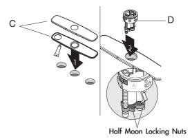
Place a bead of clear silicone sealant (not included) around the edge of the putty plate (C). Secure deck & putty plate (C) on sink or countertop. Insert base (D) into hole of deck & putty plate (C) with "FR↑NT" facing forward. Tighten screws on base (D) with 4mm hex wrench (J) until base is secure on deck & putty plate (C)
