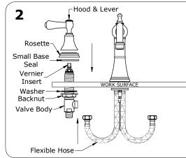
Sidevalve to be installed from underside of work surface as shown.
