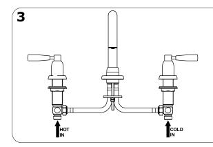
Connect and tighten the flexible hoses.
