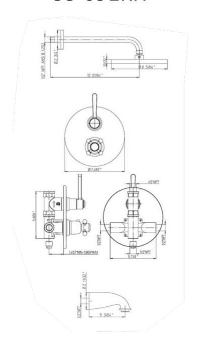
Firenze thermostatic valve with 2-way diverter volume control 8" rain shower head with 12" arm Rough included.
