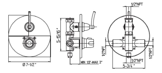
Morellino thermostatic valve with ¾" ceramic disk volume control 8" rain shower head with 12" arm ½" inlet connections Rough included.
