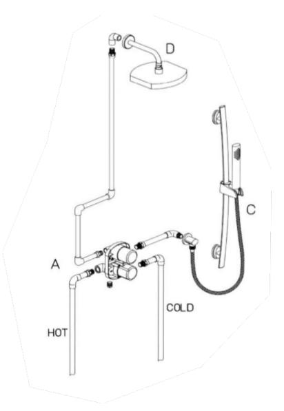
Morgana thermostatic valve with 2-way diverter volume control 8" rain shower head with 12" arm Slide bar kit Rough included.
