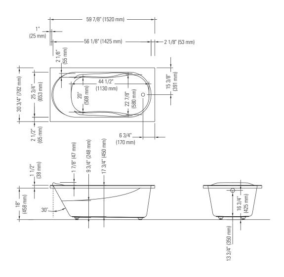
$<sup>\</sup>star$ A bathtub fitted with back jets can cause the pump to protrude by approximately 3" from the overall dimension.
