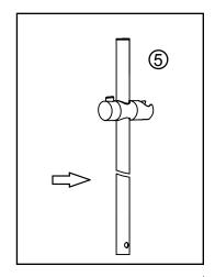
Step 4: Insert the wall bar and the slider through Holder A. Then fit the Holder B to the wall bar by tightening screws through Hole B.
