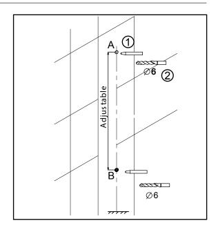
Step 2: To eject the silicons into A and B hole and then insert the wall plug. Afterwards, fix the holder A to the wall by screwing.
