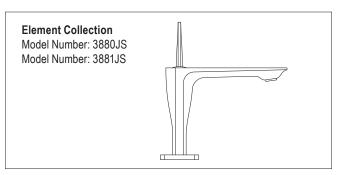
Flush both supply lines before installation, then shut off both supply lines. Minimum hole size for the spout and handle trim is 1-1/4" and maximum of 1-1/2"
