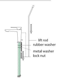
Apply a ring of silicone caulking around hole designated for spout. DO NOT USE PLUMBERS' PUTTY WHICH CAN DAMAGE FINISH. Insert faucet assembly through hole in sink or counter top, being sure to center faucet in hole.
