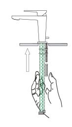
Secure fixture from below by using either an adjustable wrench, basin wrench, or deep socket to the lock nut. Wipe away excess silicone with a wet finger or damp cloth. Connect flexible hoses to their respedic water supplies.
