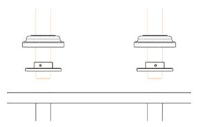
2. Mark the position of screw hole in the mounting bracket, and remove both legs. Drill the pilot holes out for the screws at 5/16".
