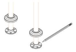
3. Wrap the threads with Teflon Tape and thread each leg into the female fittings beneath the floor.
