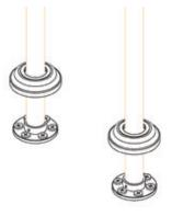
5. Wrap Teflon Tape around the threads of each leg and thread the base body onto the legs of the assembly. Use a wrench to ensure connection is tight. Being cautious to not danger the finish.
