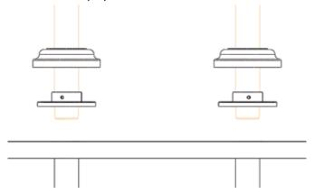
2. Mark the position of screw hole flange and remove both legs. Drill the pilot holes out for the screws at 5/16"
