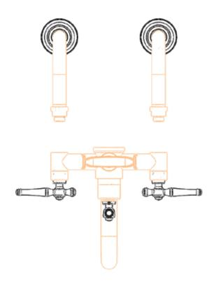
7. Place the handheld shower in the rack and thread the hose on floor mount tub filler and handheld shower respectively.
