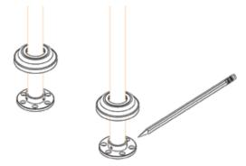
3. Wrap the threads with Teflon Tape and thread each leg into the female pipes beneath the floor.
