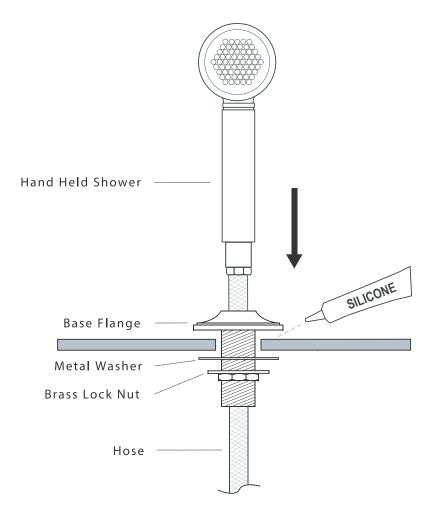
Other end of Hose to connect to Spout Diverter Valve
