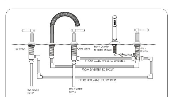
LAYOUT OF COMPLETELY INSTALLED ROMAN TUB FILLER WITH HAND HELD SHOWER
