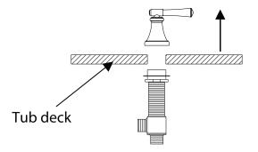
3 -Slip valve body up from below tub deck. Place the top lock nut and the fiber gasket back onto the valve body until the top surface of the lock nut is flush with the top surface of the valve body.
