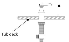
The measurements shown are for reference only. Products and specifications shown are subject to change without notice. www.santecfaucet.com | P: 310.542.0063 F: 310.542.5681 -Slip valve body up from below tub deck.
