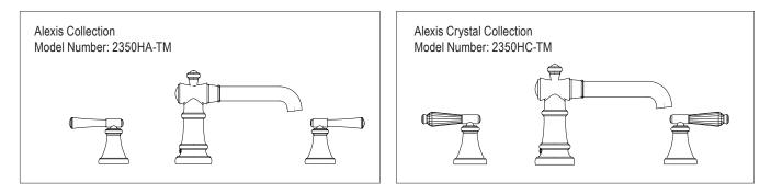
Flush both supply lines before installation, then shut off both supply lines. Minimum hole size for the spout and handle trim is 1-1/4" and maximum of 1-1/2"
