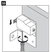
Using a screwdriver, adjust the vanity mounting hinge system counter-clockwise.
