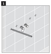
Reference the vanity specification to establish the position of mounting bolts, mark the holes to be drilled for the anchors.
