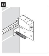
The plastic anchors provided are for concrete wall applications.
