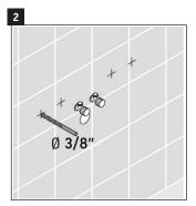
Using a 3/8" drilling bit, dirll the anchor holes that have been marked.
