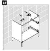
The plastic anchor provided are for concrete wall application.
