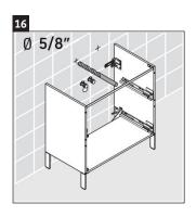
Using 5/8" drill bit, drill the anchor holes, that have been marked.
