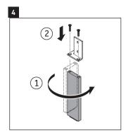
Turn leg counter-clockwise and screw two screws in.
