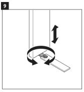
Using supplied key, adjust the legs height.
