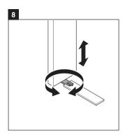
Using supplied key, adjust the legs height.
