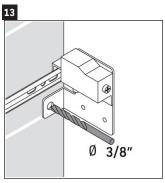
Using the appropriate bit for the wall material, dirll pilot holes.
