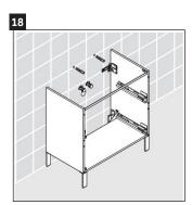
The plastic anchor provided are for concrete wall application.
