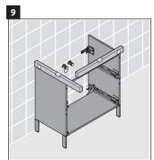
Using supplied key, adjust the legs height.
