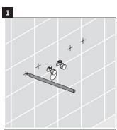
Reference the vanity specification to establish the position of mounting bolts, mark the holes to be drilled for the anchors.
