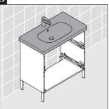
When mounting the washbasin into the wood stud wall, there must be adjustment bracing.
