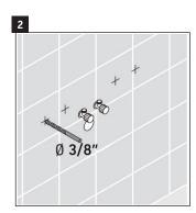
Using a 3/8" drilling bit, dirll the anchor holes that have been marked.
