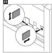
Level the vanity drawer by adjusting the two screws.
