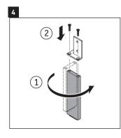
Turn leg counter-clockwise and screw two screws in.
