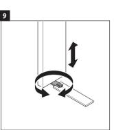
Using supplied key, adjust the legs height.
