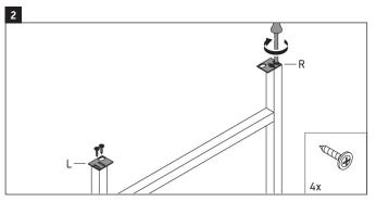
Using screw driver, screw four screws counter-clockwise.
