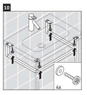
Connect the console to the washbasin using screws and washers.
