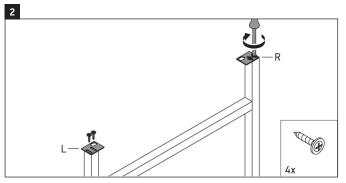
Using screw driver, screw four screws counter-clockwise.
