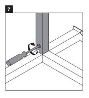
Using screw driver tighten the towel rails.
