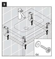
Connect the console to the washbasin using screws and washers.
