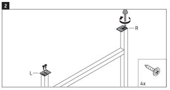
Using screw driver, screw four screws counter-clockwise. Connect smaller left and right plates with the left and right console legs.
