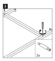
Using screw driver, screw two screws counter-clockwise.
