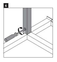
Using screw driver tighten the towel rails.
