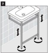
The height of the console can be adjusted by turning the bottom screws either clockwise or counter-clockwise.
