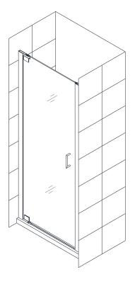
1. Place the **Wall profile for glass door (01)** on the shower base or the threshold vertically against the finished wall.
