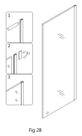
27. Place the **Wall profile for glass door (01)** on the shower base or the threshold vertically against the finished wall. Adjust the **Wall profile for glass door** vertically using a level.
