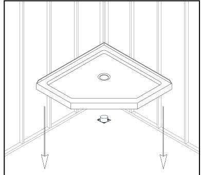
Lower the base over the drain pipe and set it into place against the studs.
