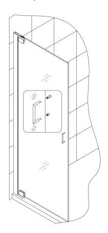
34. Press the **Anti-water strip (29)** onto the vertical edge of the **Stationary glass (21)**.
