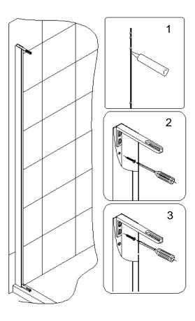
4. Attach the **Pivot assembly (07)** to the top and the bottom ends of the **Glass profile for glass door (02)** with the **Flat head screws ST4.2×25 (15)** and **M4×16 bolt (13)**.
