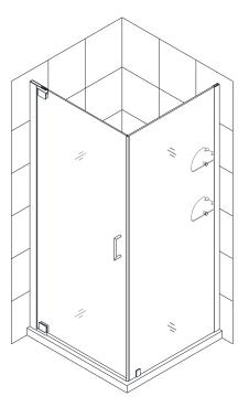
Mark the Glass shelf (22) position on the wall. According to the measurements in Fig. 46.1, mark the drilling holes for the Shelf brackets (without nut) (31).
