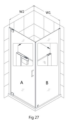
26. Apply clear silicone along the inner channel of the **Glass profile (04)** and push the **Stationary glass (21)** inside the channel.
