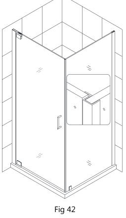
40. After final adjustments of the **Assembled unit** drill the holes in the **Glass profiles (02)** and **(04)** through predrilled holes in the **Wall profiles (01)** and **(05)** using **Ø 1/8**" drill bit.
