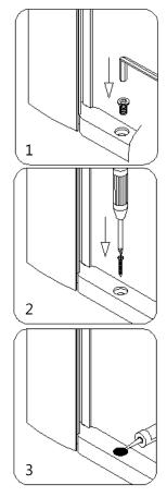
39. Do the final adjustment if necessary. Make sure the **Glass door (03)** closes tight to the **Anti-Water strip** (29).
