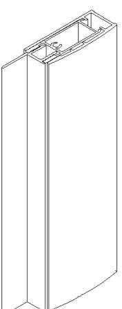
12. Use a level to ensure that the **Glass door (03)** and the **Wall profile (05)** is absolutely vertical. Draw a line along the vertical edge of the **Wall profile** on the wall. Detach the **Wall profile** from the **Glass profile (04).** Place the **Wall profile** to the outlined position and mark the drilling holes through the predrilled holes in the **Wall profile.**
