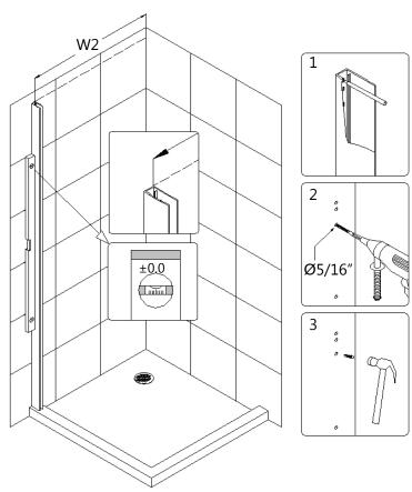
28. Push the **Pivot retainers (08)** into both ends of the **Wall profile for glass door (01)**.
