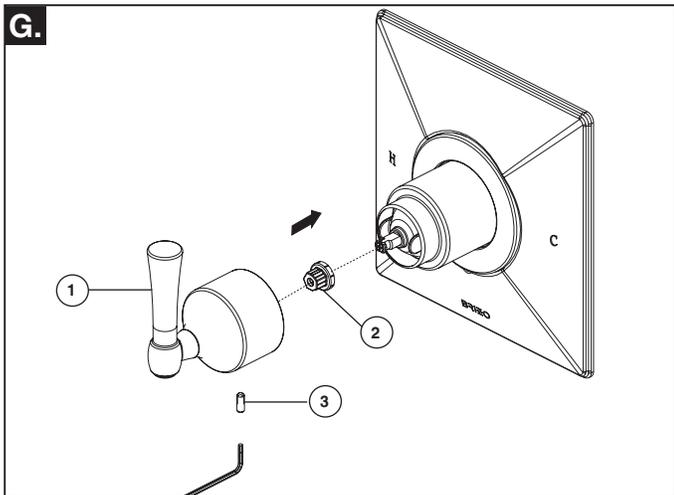
**G.** Push insert (1) onto the stem and install handle (2) onto the insert, tighten set screw (3) to secure handle.
