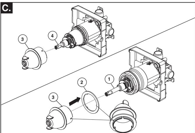
**C.** If you are using the 1 3/4" stem extender (1), slide the adapter ring (2) into the grooves at the bottom of the guide (3). Slide the guide (3) over the stem until the ring rests on the bonnet. If you are using the 1" stem extender (4), you will not need the adapter ring.
