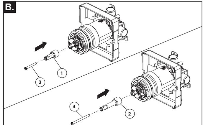
**B.** Decide if 1" extension (1) or 1 3/4" extension (2) is needed. Place extender onto cartridge stem and secure in place using appropriate screw (3) or (4).
