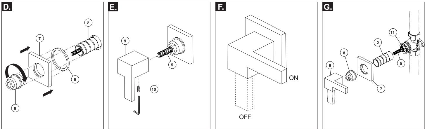
**D.** Install gasket (6) onto the back of escutcheon (7). Slide escutcheon over the extension sleeve (2) and tighten with bonnet nut (8). Do not over-tighten.
