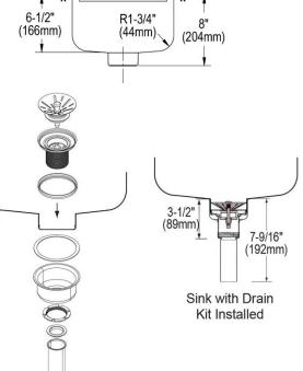
Sink with Drain Kit Installed
