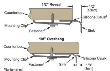
Designed to affix to the underside of any solid surface countertop.
