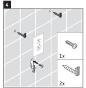
Thread the two mounting screws into top two anchors, leaving hooks facing up. Secure the L-bracket to wall with set screw on the bottom.
