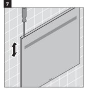
Use adjustment tool to move mirror up and down for leveling.
