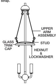
11) Align (1) of remaining arms from top tier to hole in strap and thru trim. Pass stud thru hole in strap and keyhole of trim. Slip lockwasher on stud and thread hexnut on stud. Tighten to secure. Repeat for opposite arm.
