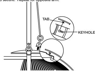
12) Remove hexnut and lockwasher from (1) arm attached to glass trim from step 12. Align metal tab on bottom side of strap to larger end of keyhole. Pass tab thru keyhole and slide downward to bottom end of keyhole. Align upper tier arm with loop and pass stud thru hole in strap and keyhole of trim. Slip lockwasher on stud and thread hexnut on stud. Tighten to secure. Repeat for opposite side.
