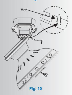
Step 3. Carefully feed the electrical lead wires from the fan up through the downrod. Thread the downrod into the coupling until the Hitch pin holes are aligned.
