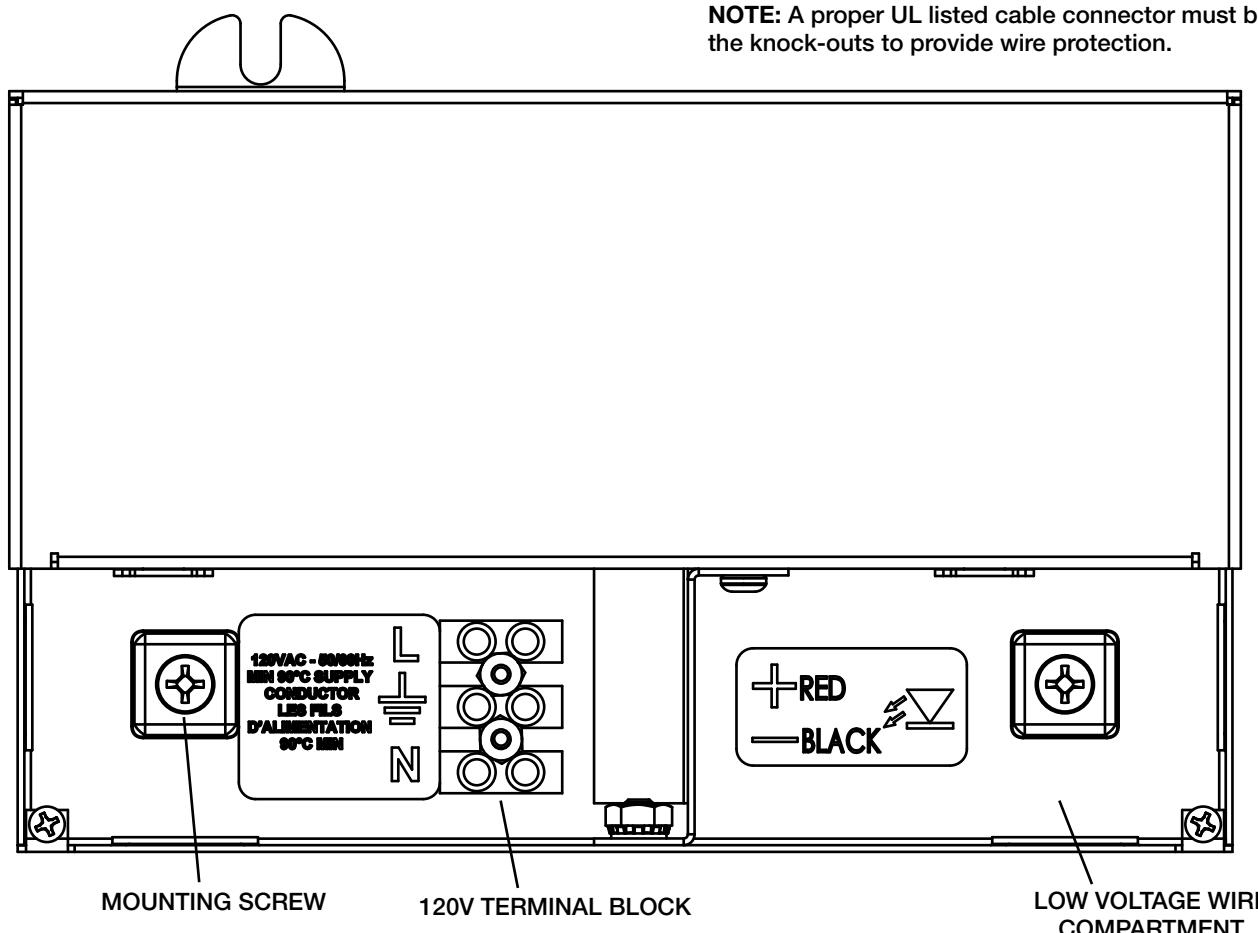
**NOTE:** Kichler 6TL-Series (24V) and 4TL-Series (12V) Power Supplies are not compatible with dimmers when used in conjunction with tape light controllers.
