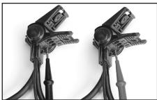
STEP 4 (Optional if testing voltage at fixture) Turn power back on. With connector still open halfway, push voltmeter probe into connector probe port. Push probe all the way in and repeat on other connector.
