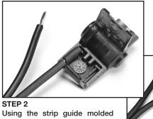
into the connector for reference, strip the wire to 11/16".
