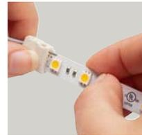
4. Remove 3M backing from tape light and apply making sure to press between the LED's and other components. **Pressing on the LED's and other components will result in damage to the tape.**
