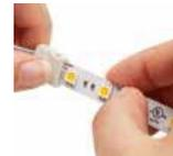
4. Remove 3M backing from tape light and apply making sure to press between the LED's and other components. **Pressing on the LED's and other components will result in damage to the tape.**
