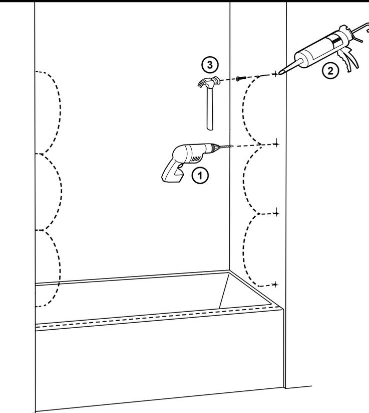
**5 SECURE WALL JAMB ON THE SIDE WHERE THE DOOR WILL CLOSE / SÉCURISER LE JAMBAGE DU CÔTÉ DE LA FERMETURE DE PORTE**
