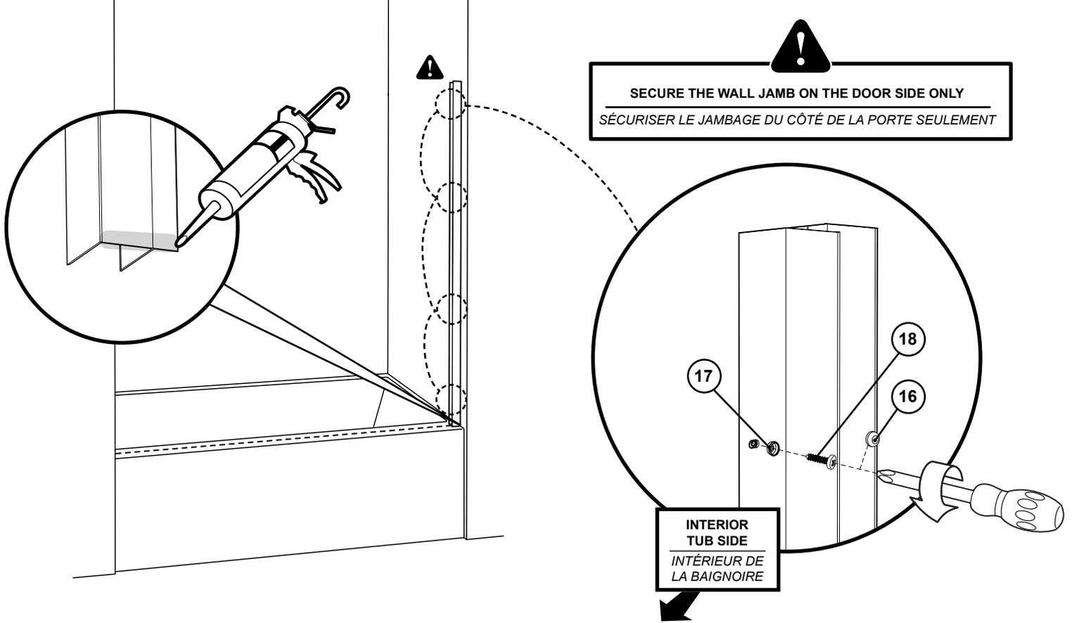
**6 ASSEMBLE THE FRAME / ASSEMBLER LE CADRE**
