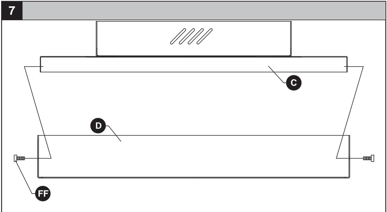
7. Raise shade (D) to the LED housing (C) and secure with shade screw (FF).
