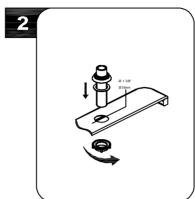
Insert body assembly through selected hole in sink. Secure body to sink by screwing the mounting nut from the underside of the sink. Hand tighten only.
