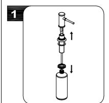
Remove the bottle. Separate soap dispenser head from flange body assembly.
