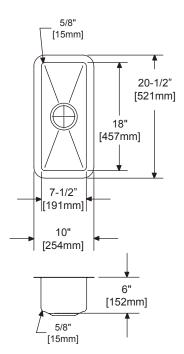
Installation Profile of EFRU Models The template provided with each EFRU sink provides the only type of installation recommended by Elkay.
