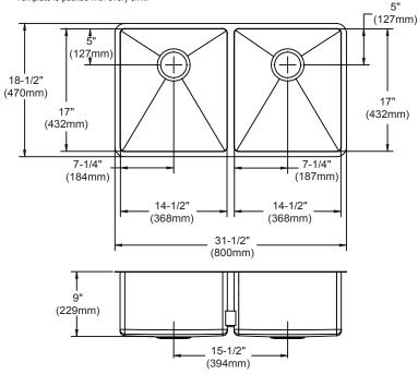
Installation Profile of ECTRU Models
