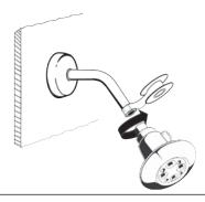
**2** Remove any excess materials left on the threads of the shower arm and wrap plumber tape around the threads.
