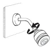
3 Hand tighten the new shower head to the shower arm by turning clock wise. Turn on the water and check the system for leaks.
