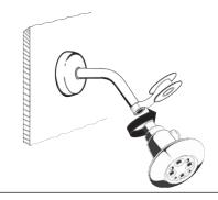
**2** Remove any excess materials left on the threads of the shower arm and wrap plumber tape around the threads.
