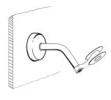
**4** To adjust the water flow, set desired water flow by turning the knob.
