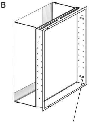
Hinge Plate shown for right hinged door. Handed door is determined at the time of order. Be sure to install with left or right hinged unit on the correct side.
