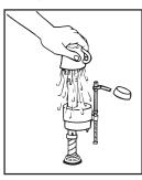
While holding a container over the uncapped VALVE to prevent splashing, turn water supply on and off a few times. Leave water supply off.
