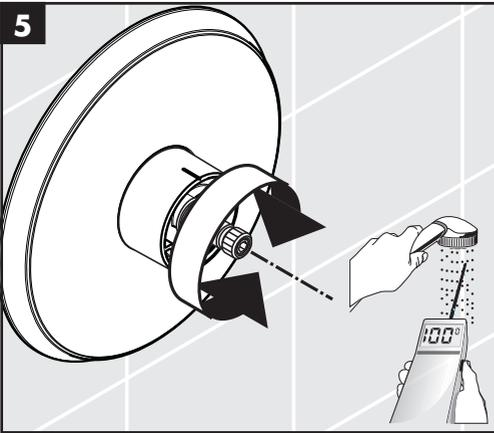
Install the handle so that the override button is next to the 100° mark.
