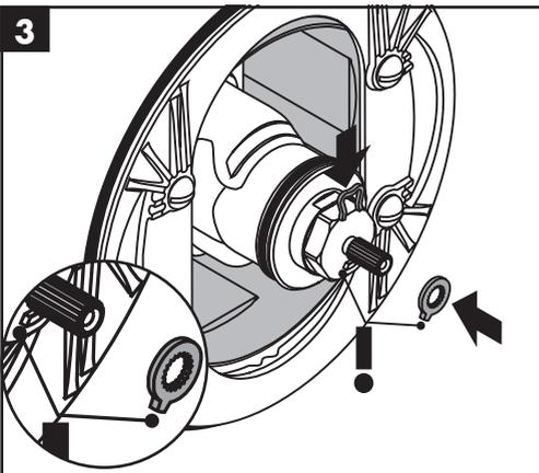
Replace the stop ring so that the tooth is against the cartridge stop. Replace the clip.
