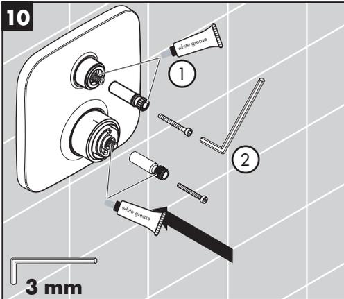
Lubricate the adapter stems with a small amount of white plumber's grease (1).
