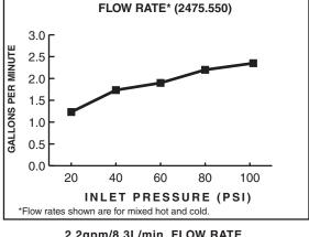
2.2gpm/8.3L/min. FLOW RATE
