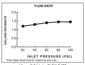
1.5gpm/5.7 L/min. FLOW RATE
